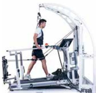
gait symmetry with bio-feedback left vs. right and on-line active gait correction with robowalk
