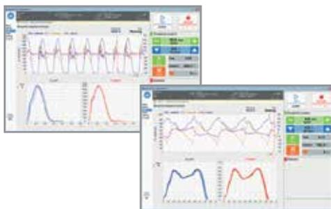
3 component force measurement,  $F_z$ ,  $F_y$ ,  $F_x$  during running (left) and walking (right) on the gaitway<sup>®</sup> 3d
