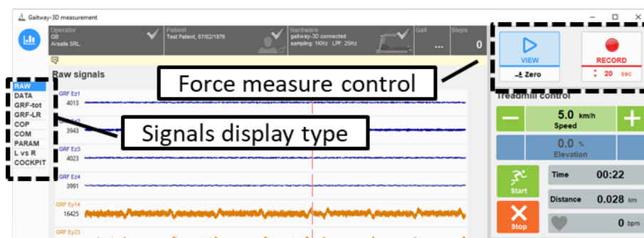
Figure 19: gaitway-3D software measure screen: Force measure control and display
