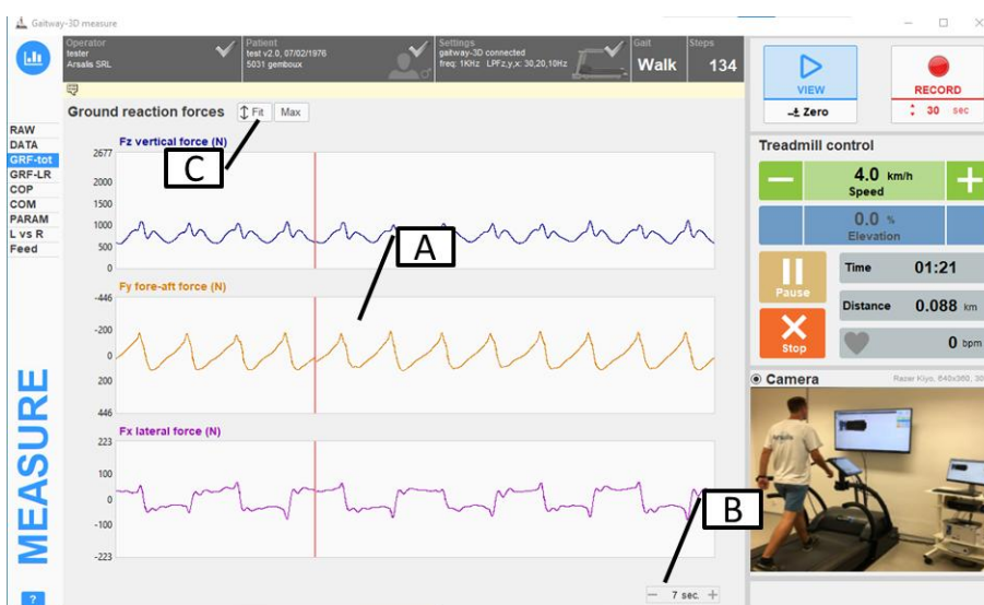
Figure 22: gateway-3D software measure screen: Ground reaction forces.
